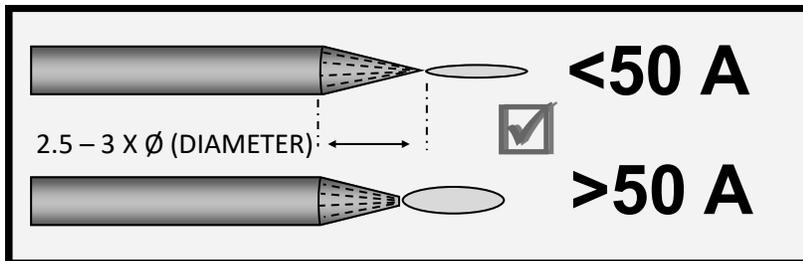
Use a point for low amp use to help control arc. Create a slight truncation on the tip for higher amp use for best arc stability. Grind the tip so that it is 2.5- 3 times longer than the tungsten is wide (Diameter).
