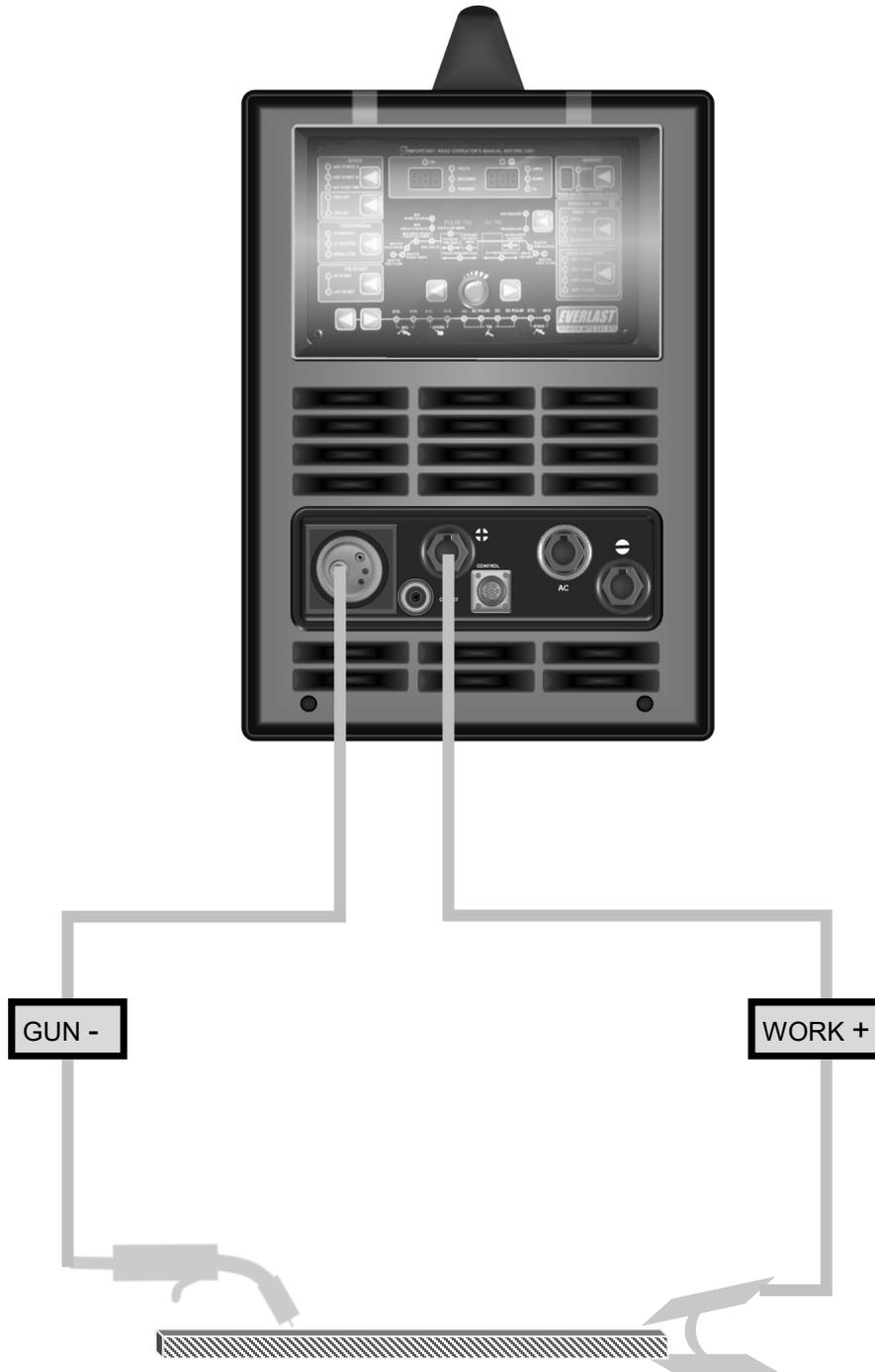
\*The feeder connection located under the spool cover must be located on the negative terminal. Flux-Core wire requires that the gun be used electrode negative (EN) in most cases. Consult the wire manufacturer recommendations as the final authority. Dual shield wire is run
