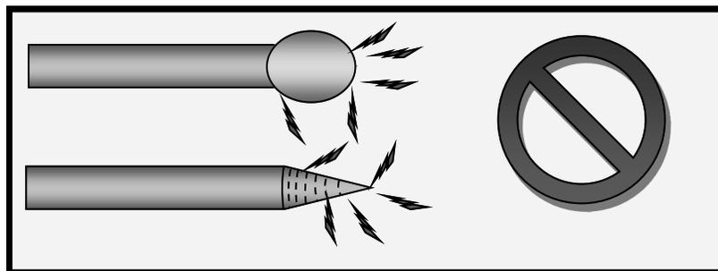
Do not ball the Tungsten while welding, or an erratic arc will result. Make sure that the grinding marks run parallel to the tip. Concentric marks will also cause an erratic arc.
