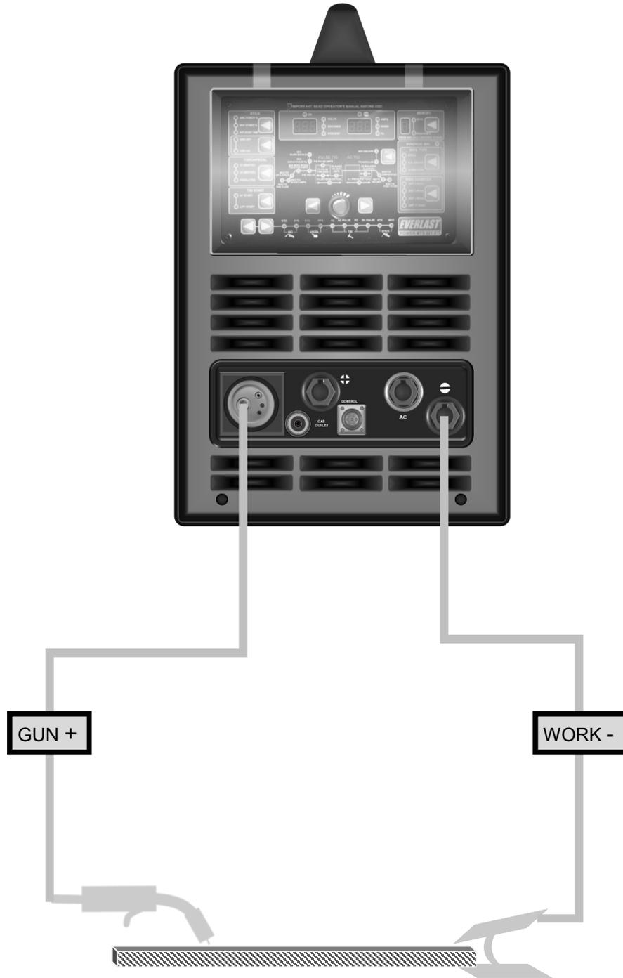
\*The feeder connection located under the spool cover must be located on the positive terminal. MIG requires that the gun be used with a positive polarity.
