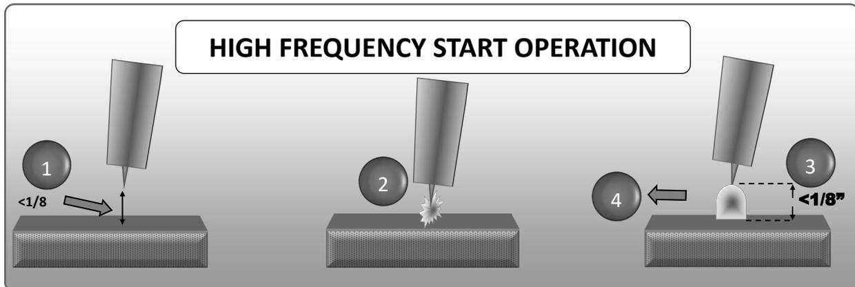
1. Position the point of the sharpened tungsten about 1/8" or less above the metal.
